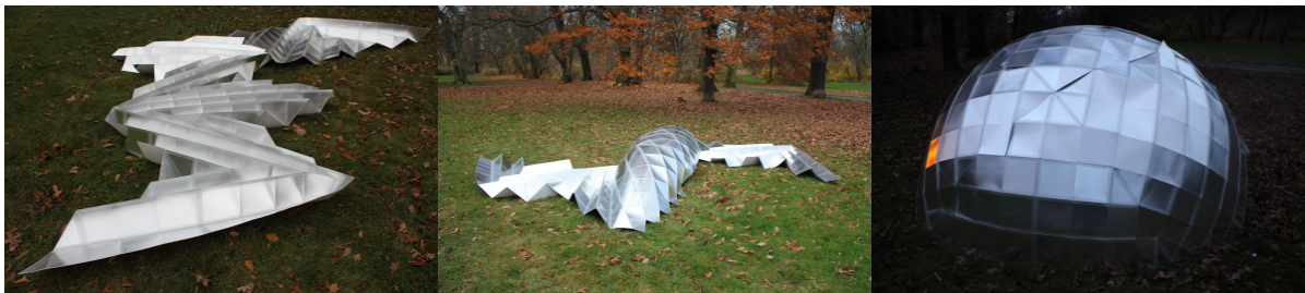
Figures 4 to 6: Unfolding process of a 5 frequency dome
